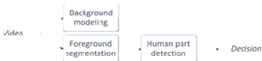
Figure 13. Block diagram of the proposed system for a general video input.
